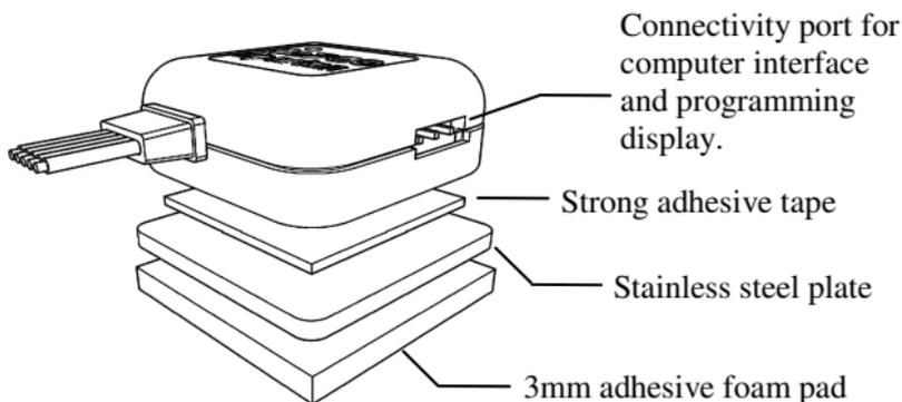
**Important:** Do not mount the gyro in locations where it may be subjected to high levels of oily smoke, fuel, or other liquids. Do not allow the cable to touch the sharp edge of the helicopter frames as over time the cable insulation may be damaged. Inspect the condition of the adhesive pads as part of your regular pre-flight checks.
