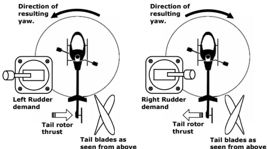
When performing the final checks of the gyro installation, you should also check the correct operation of the gyro direction. To do this set the
