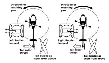
When performing the final checks of the ds760 installation, you should also check the correct operation of the gyro direction. To do this set the
